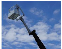
\* This extension is rated as non-insulated and not intended for energized work
